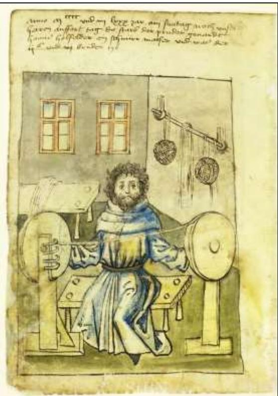
Twisting yarns into rope
