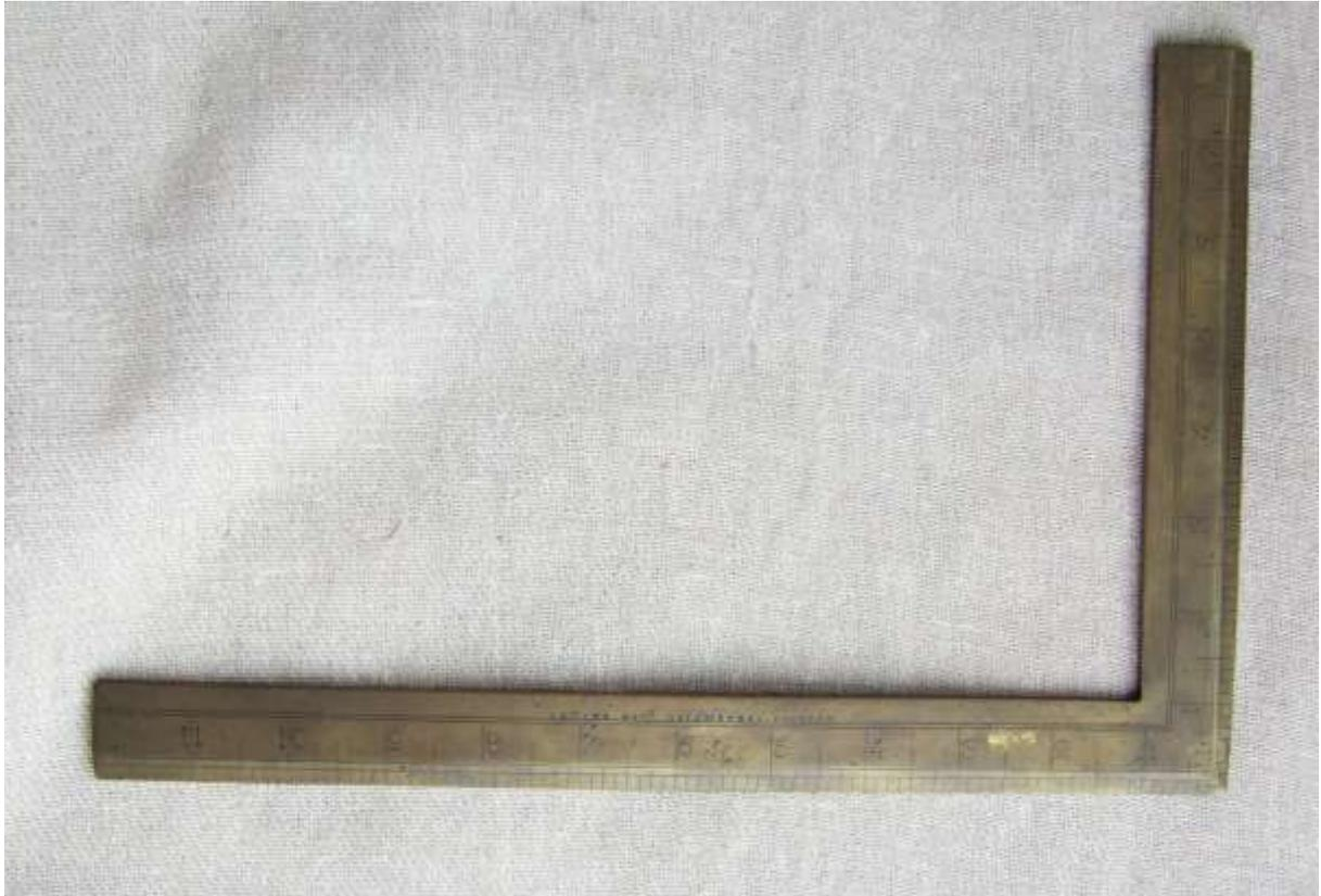
This brass square, with 12 inch and 9 inch arms, marked *Sadler Bros Sailmakers Ipswich*, is slightly curious, as the square is not regularly mentioned as a tool of the sailmaking trade, although it could be used in laying out and cutting the panels of canvas. If not all wood, brass would be an ideal material to work on canvas that may have been salt laden, but one especially marked is certainly very unusual.
